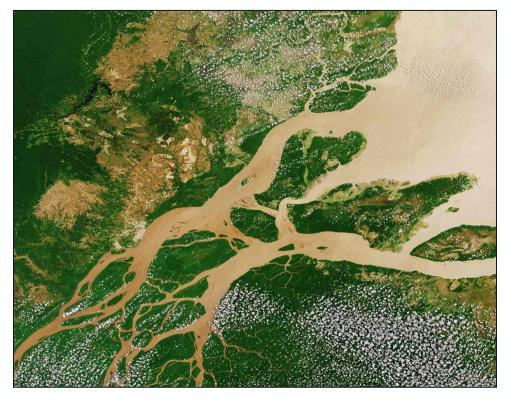
Sediment discharge of the Amazon River congregates into mud banks captured by Sentinel-2. Sediments are migrated by forces of waves and currents westward along the northeast South America coastline.
