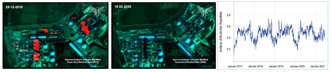
Cement plant activity index for China generated using Sentinel-2 data. The index represents the utilization rate of a country's production capacity, equal to the average utilization rate of each cement plant, weighted by its capacity.
